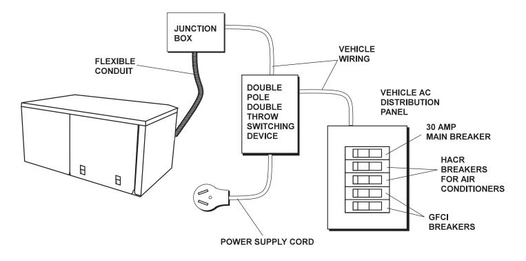
Figure 2.15 – Installation With Isolation Receptacle
